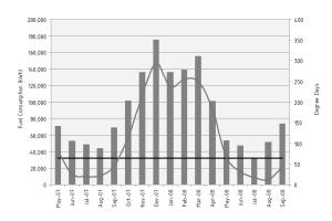
Figure 1: Monthly gas fuel consumption and degree days for Hounslow health centre (Source: Daniela Skarica, student, 2008)
